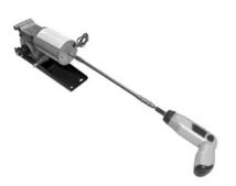
If the cables tighten, and the motor is difficult to turn, REVERSE THE DIRECTION. OVER-TORQUEING CAN HAPPEN, RESULTING IN SEVERE DAMAGE.
