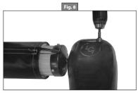
□ Using a 7/16" nut driver and power drill, spin the manual override nut counterclockwise to retract the awning (**Fig 8**). A 7/16" socket and ratchet can be used if a drill is not available.
